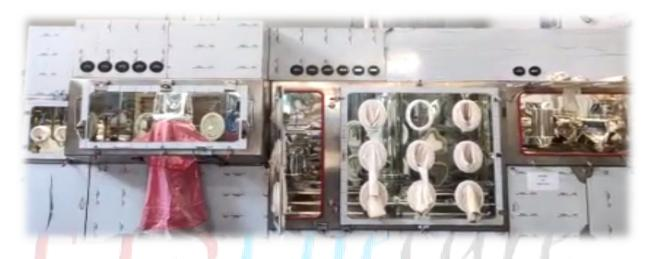
This Granulator machine is a one smart unit for all operations and comprises of different sections including sifting, wet high shear mixing and granulating, co-milling, drying and blending of small batches of up to 10 kg batch size.
